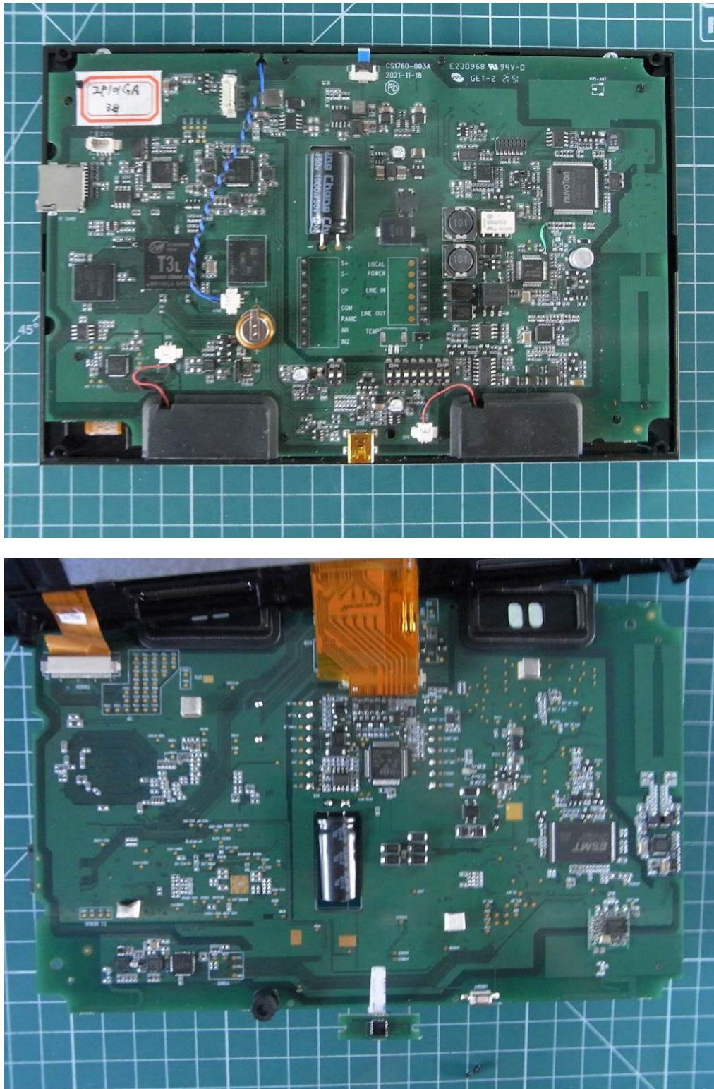
**EUT IDENTIFICATION – Internal views – 13.56 MHz radio module and antenna**
