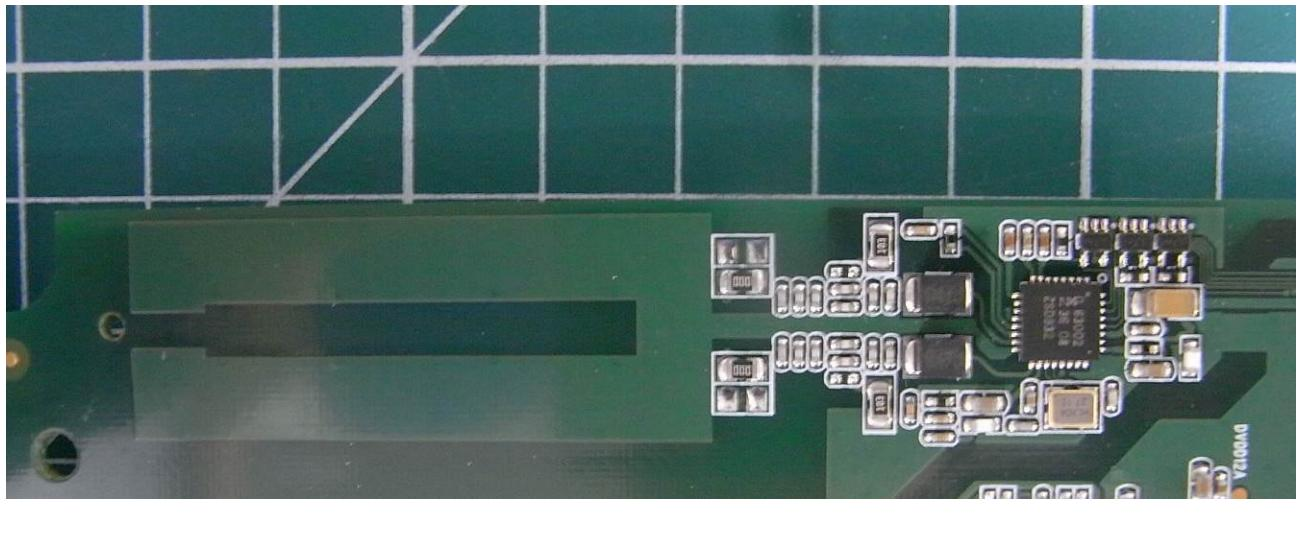
**EUT IDENTIFICATION – Internal views – Wi-Fi radio module and antenna**
