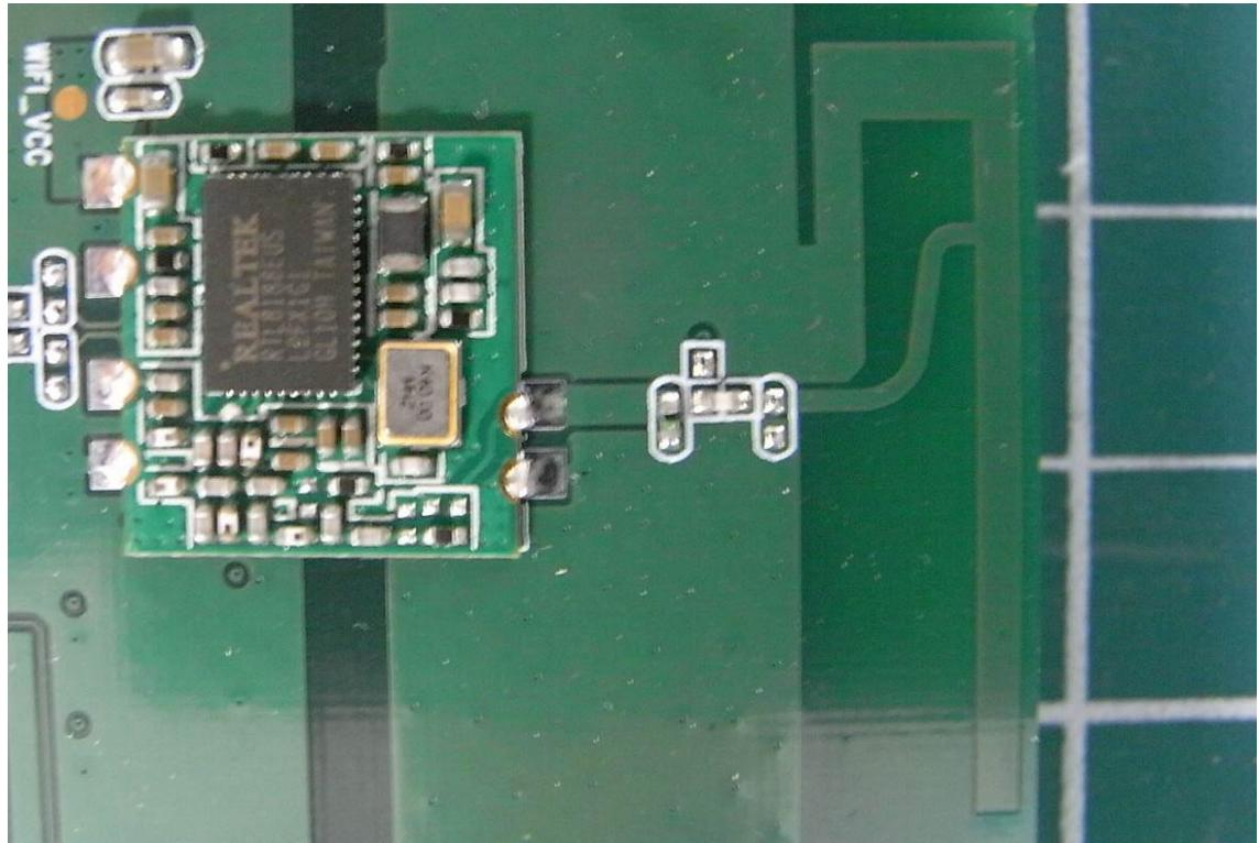
**EUT IDENTIFICATION – Internal views – 13.56 MHz radio module and antenna**
