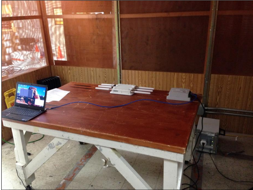
Photograph 5. Conducted Emissions, 15.207(a), Test Setup, with PowerDsine9501GO
