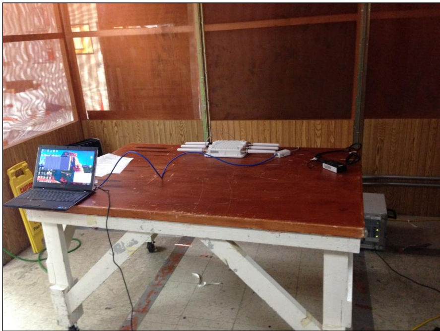
Photograph 2. Conducted Emissions, Test Setup, with FSP Power Supply
