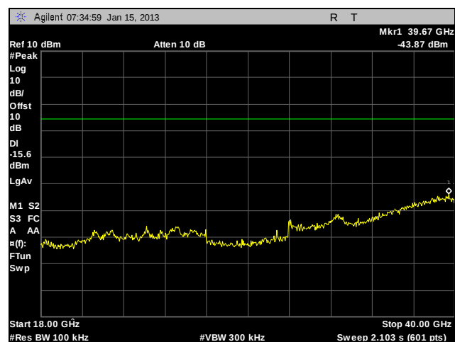
Plot 416. Conducted Spurious Emissions, 802.11n 40 MHz, 5755 MHz, Low Channel, Port 2, 18 GHz - 40 GHz
