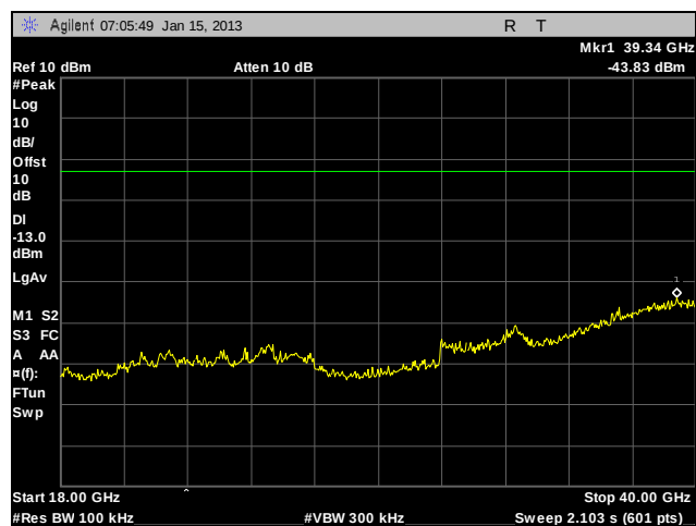
Plot 407. Conducted Spurious Emissions, 802.11n 20 MHz, 5805 MHz, High Channel, Port 3, 18 GHz - 40 GHz
