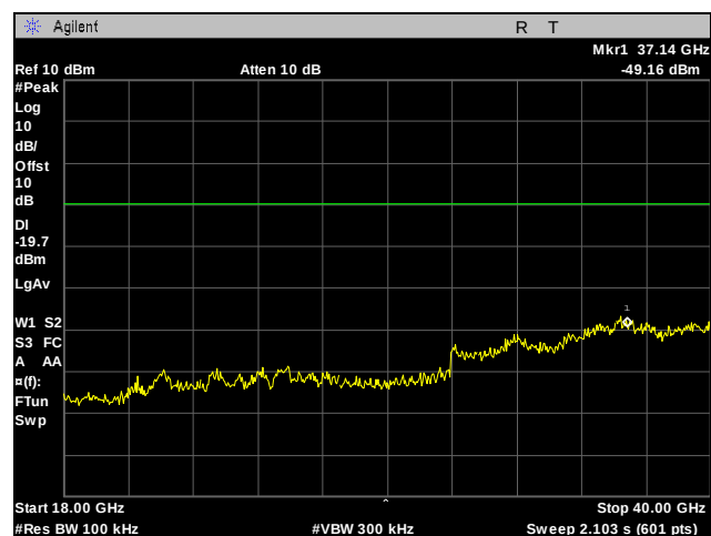
Plot 428. Conducted Spurious Emissions, 802.11n 80MHz, 5775 MHz, Port 1, 18 GHz - 40 GHz
