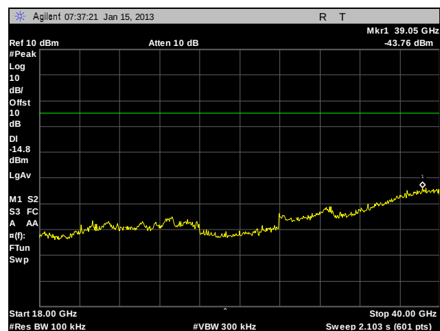
Plot 422. Conducted Spurious Emissions, 802.11n 40 MHz, 5755 MHz, Low Channel, Port 3, 18 GHz - 40 GHz
