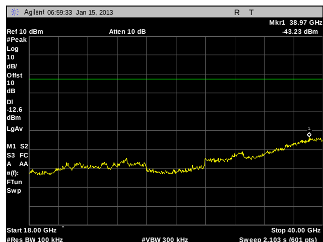
Plot 401. Conducted Spurious Emissions, 802.11n 20 MHz, 5745 MHz, Low Channel, Port 3, 18 GHz - 40 GHz
