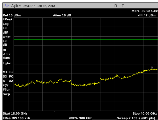
Plot 380. Conducted Spurious Emissions, 802.11a, 5805 MHz, High Channel, Port 1, 18 GHz - 40 GHz
