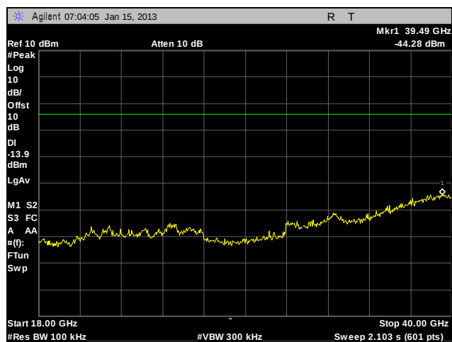
Plot 404. Conducted Spurious Emissions, 802.11n 20 MHz, 5785 MHz, Mid Channel, Port 3, 18 GHz - 40 GHz
