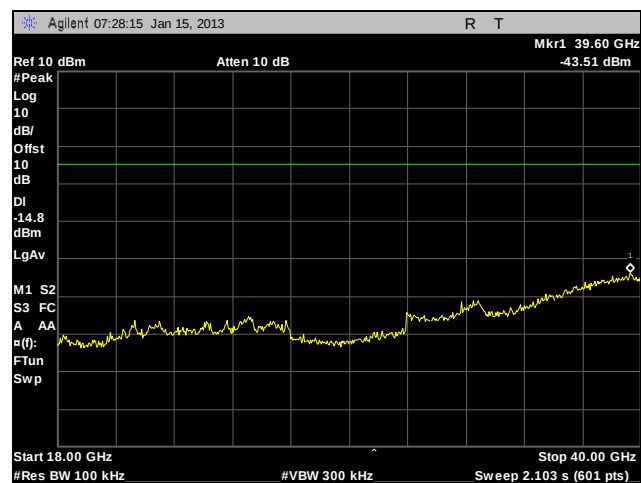
Plot 377. Conducted Spurious Emissions, 802.11a, 5785 MHz, Mid Channel, Port 1, 18 GHz - 40 GHz
