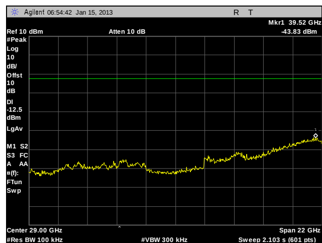
Plot 392. Conducted Spurious Emissions, 802.11n 20 MHz, 5745 MHz, Low Channel, Port 2, 18 GHz - 40 GHz
