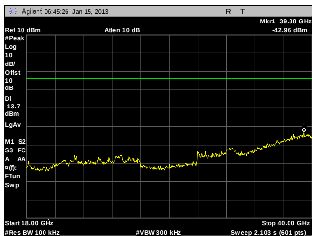
Plot 386. Conducted Spurious Emissions, 802.11n 20 MHz, 5785 MHz, Mid Channel, Port 1, 18 GHz - 40 GHz
