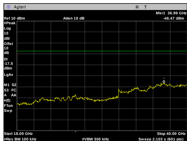
Plot 434. Conducted Spurious Emissions, 802.11n 80MHz, 5775 MHz, Port 3, 18 GHz - 40 GHz
