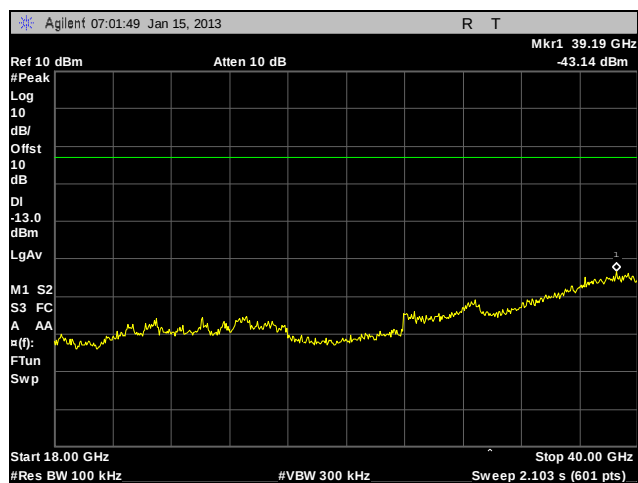
Plot 395. Conducted Spurious Emissions, 802.11n 20 MHz, 5785 MHz, Mid Channel, Port 2, 18 GHz - 40 GHz
