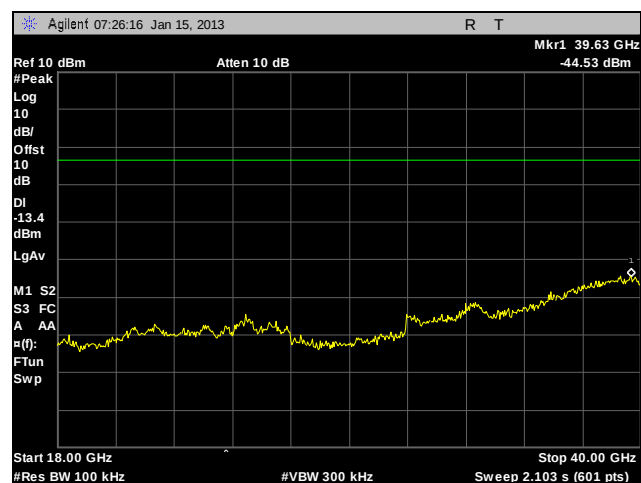
Plot 374. Conducted Spurious Emissions, 802.11a, 5745 MHz, Low Channel, Port 1, 18 GHz - 40 GHz
