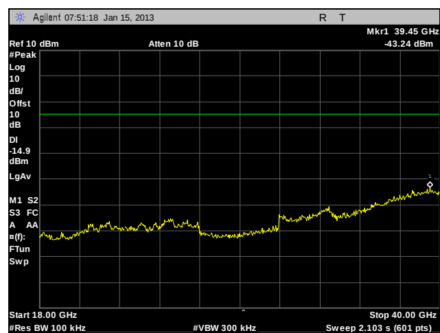
Plot 413. Conducted Spurious Emissions, 802.11n 40 MHz, 5795 MHz, High Channel, Port 1, 18 GHz - 40 GHz
