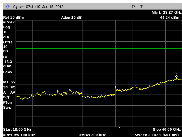
Plot 419. Conducted Spurious Emissions, 802.11n 40 MHz, 5795 MHz, High Channel, Port 2, 18 GHz - 40 GHz
