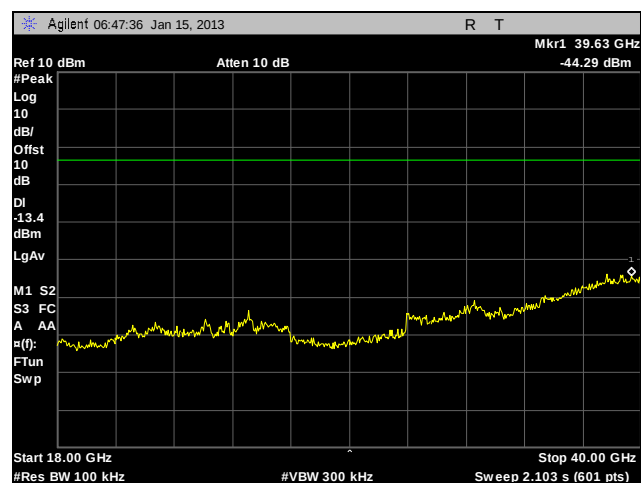
Plot 383. Conducted Spurious Emissions, 802.11n 20 MHz, 5745 MHz, Low Channel, Port 1, 18 GHz - 40 GHz
