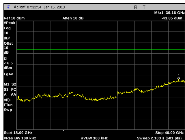
Plot 410. Conducted Spurious Emissions, 802.11n 40 MHz, 5755 MHz, Low Channel, Port 1, 18 GHz - 40 GHz
