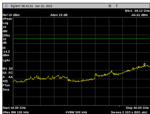
Plot 389. Conducted Spurious Emissions, 802.11n 20 MHz, 5805 MHz, High Channel, Port 1, 18 GHz - 40 GHz
