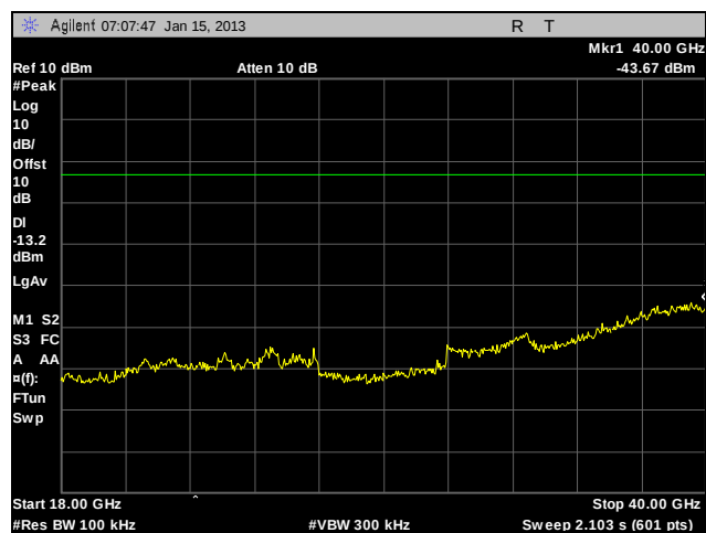
Plot 398. Conducted Spurious Emissions, 802.11n 20 MHz, 5805 MHz, High Channel, Port 2, 18 GHz - 40 GHz
