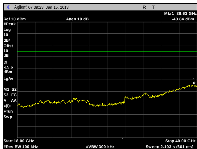
Plot 425. Conducted Spurious Emissions, 802.11n 40 MHz, 5795 MHz, High Channel, Port 3, 18 GHz - 40 GHz
