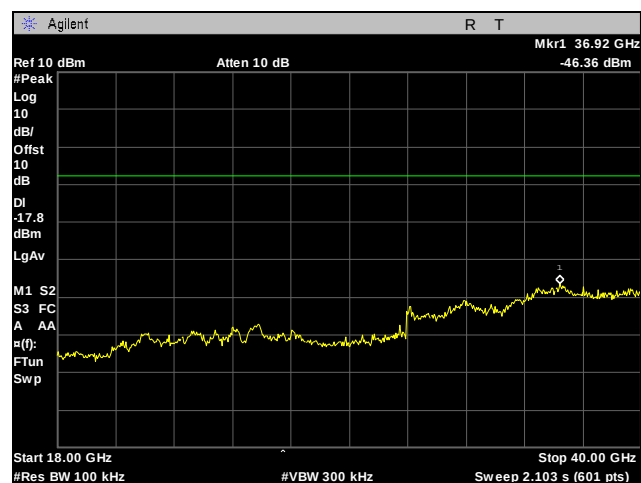
Plot 431. Conducted Spurious Emissions, 802.11n 80MHz, 5775 MHz, Port 2, 18 GHz - 40 GHz
