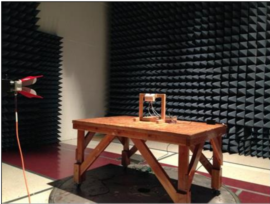
Photograph 6. Radiated Spurious Emissions, Test Setup, Above 1 GHz, Ceiling Antenna
