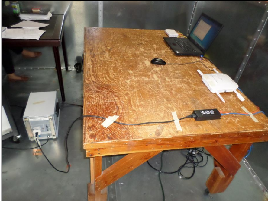
Photograph 1. Conducted Emissions, Test Setup, PoE
