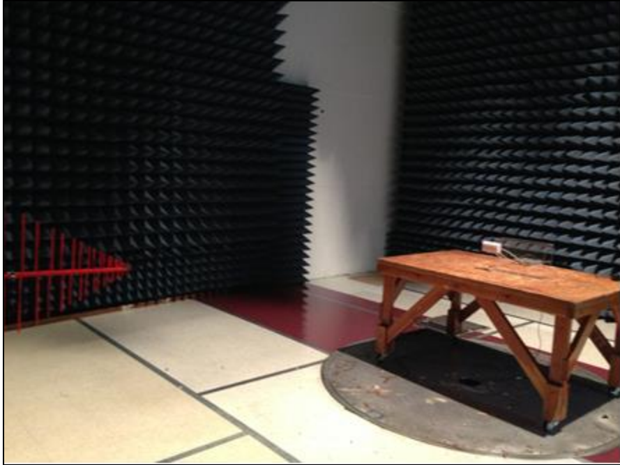
Photograph 5. Radiated Spurious Emissions, Test Setup, 30 MHz – 1 GHz, Ceiling Antenna
