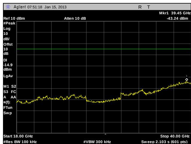
Plot 672. Conducted Spurious Emissions, 802.11n 40 MHz, 5795 MHz, High Channel, Port 1, 18 GHz - 40 GHz
