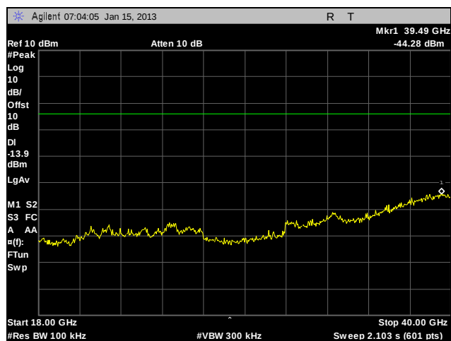
Plot 663. Conducted Spurious Emissions, 802.11n 20 MHz, 5785 MHz, Mid Channel, Port 3, 18 GHz - 40 GHz
