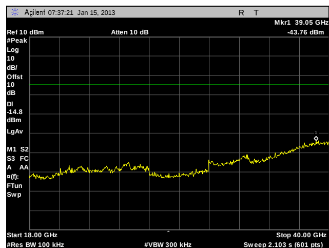
Plot 681. Conducted Spurious Emissions, 802.11n 40 MHz, 5755 MHz, Low Channel, Port 3, 18 GHz - 40 GHz
