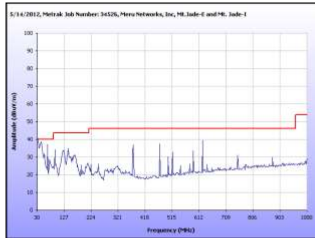
Plot 124. Radiated Spurious Emissions, 802.11n 40 MHz, Low Channel, 30 MHz – 1 GHz
