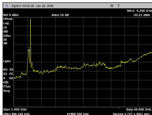
Plot 344. Conducted Spurious Emissions, Low Channel, 1 GHz – 40 GHz, 802.11n HT40, Port 3, 5 GHz
