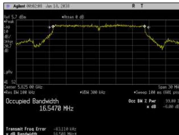
Plot 62. 6 dB Occupied Bandwidth, High Channel, 802.11a, 5 GHz
