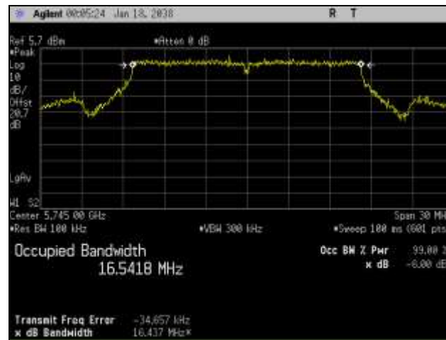
Plot 60. 6 dB Occupied Bandwidth, Low Channel, 802.11a, 5 GHz
