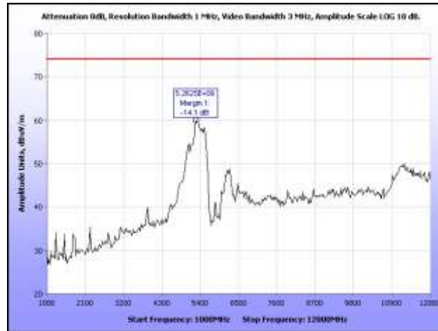
Plot 224. Radiated Spurious Emissions, High Channel, 802.11n HT20, 1 – 12 GHz, Peak, 5 GHz
