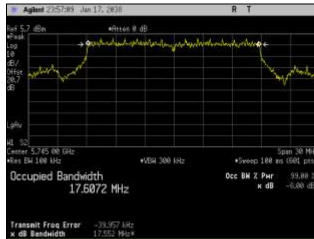
Plot 63. 6 dB Occupied Bandwidth, Low Channel, 802.11n HT20, Port 1, 5 GHz
