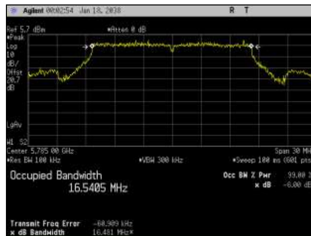
Plot 61. 6 dB Occupied Bandwidth, Mid Channel, 802.11a, 5 GHz
