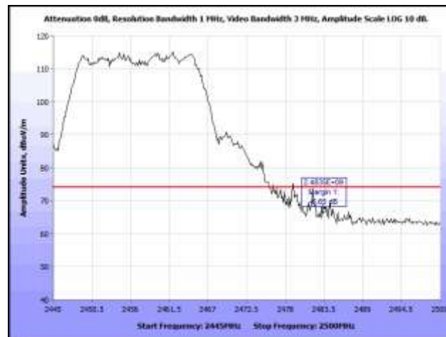
Plot 398. Radiated Band Edge, 802.11n HT20, Channel 10, 6 dBi Patch, Peak, 2.4 GHz
