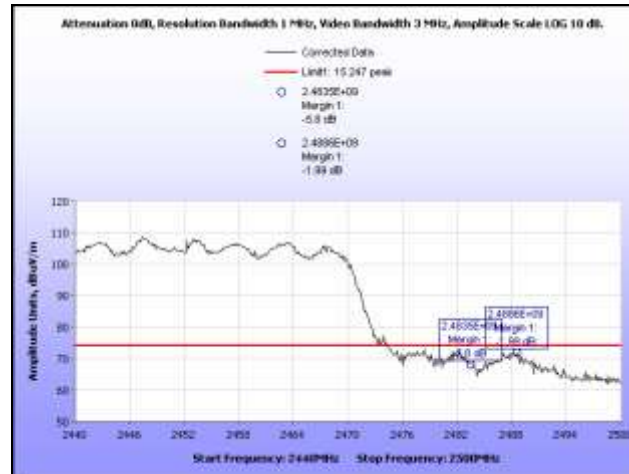
Plot 444. Radiated Band Edge, 802.11n HT40, High Channel, 3 dBi Ceiling Mount Omni, Peak, 2.4 GHz
