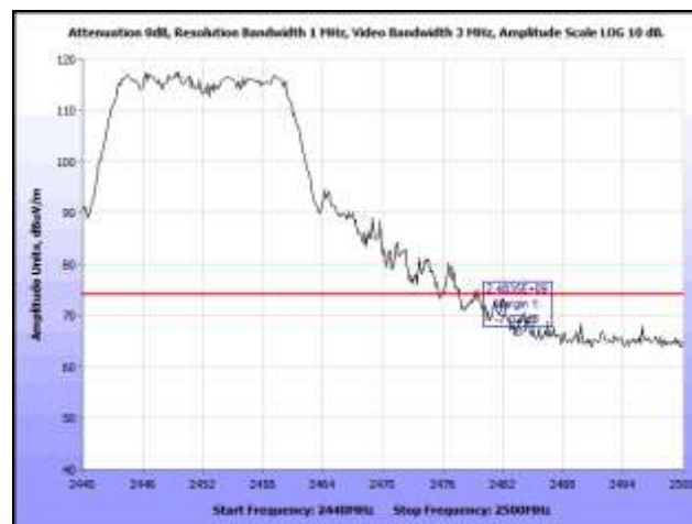
Plot 396. Radiated Band Edge, 802.11n HT20, Channel 9, 6 dBi Patch, Peak, 2.4 GHz
