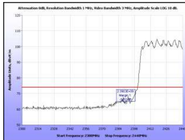
Plot 430. Radiated Band Edge, 802.11n HT40 Low Channel, 3 dBi Ceiling Mount Omni, Peak, 2.4 GHz
