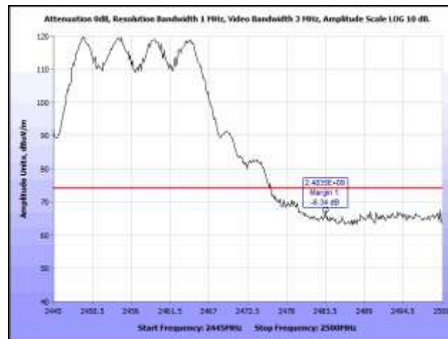
Plot 366. Radiated Band Edge, 802.11n HT20, Channel 10, 6 dBi Omni, Peak, 2.4 GHz
