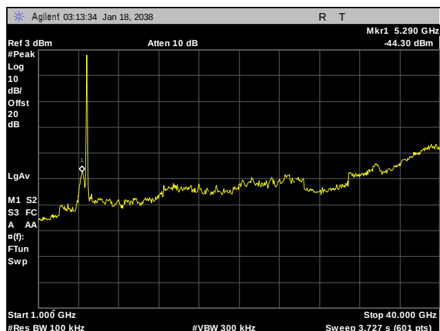
Plot 518. Conducted Spurious Emissions, Low Channel, 1 GHz – 40 GHz, 802.11n HT40, Port 1, 5 GHz
