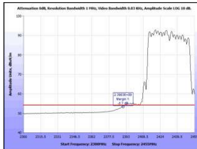
Plot 405. Radiated Band Edge, 802.11n HT40, Channel 5, 6 dBi Patch, Avg., 2.4 GHz
