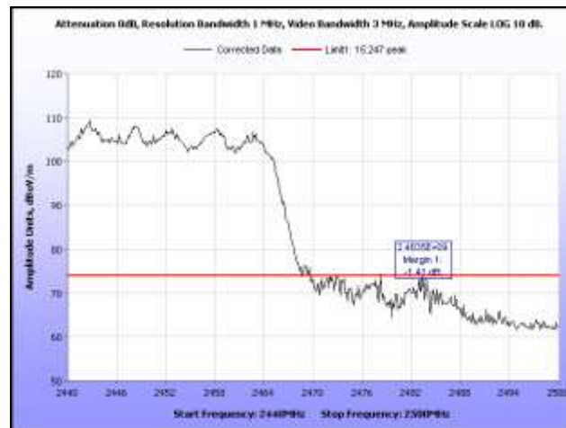
Plot 442. Radiated Band Edge, 802.11n HT40, Channel 8, 3 dBi Ceiling Mount Omni, Peak, 2.4 GHz
