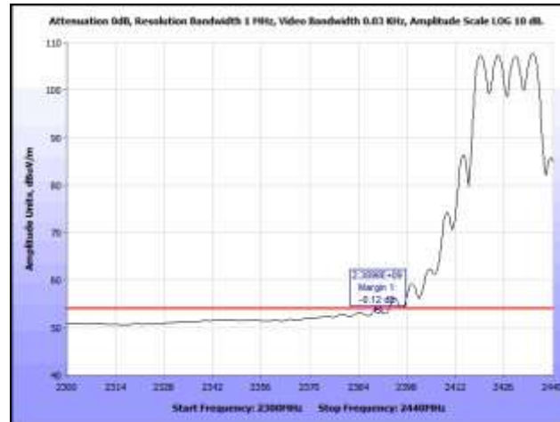
Plot 359. Radiated Band Edge, 802.11n HT20, Channel 4, 6 dBi Omni, Avg., 2.4 GHz
