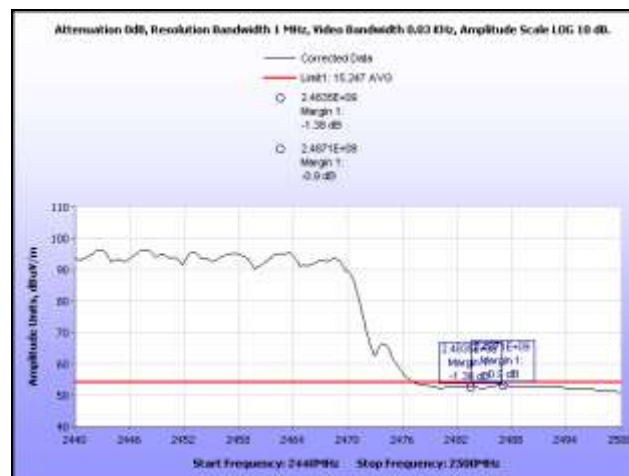
Plot 443. Radiated Band Edge, 802.11n HT40, High Channel, 3 dBi Ceiling Mount Omni, Avg., 2.4 GHz
