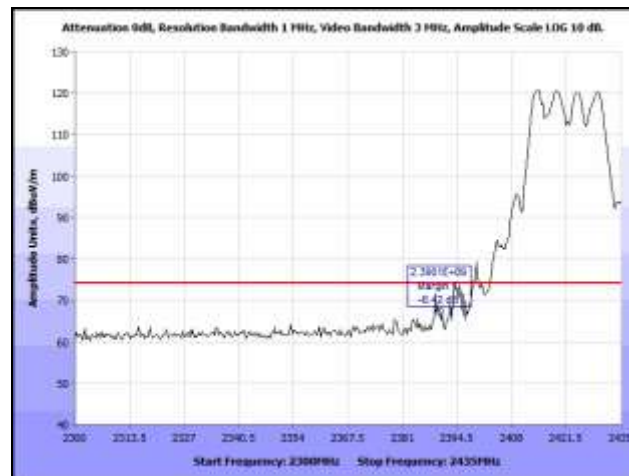
Plot 358. Radiated Band Edge, 802.11n HT20, Channel 3, 6 dBi Omni, Peak, 2.4 GHz
