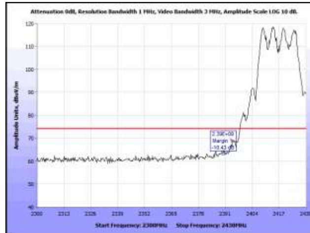
Plot 356. Radiated Band Edge, 802.11n HT20, Channel 2, 6 dBi Omni, Peak, 2.4 GHz
