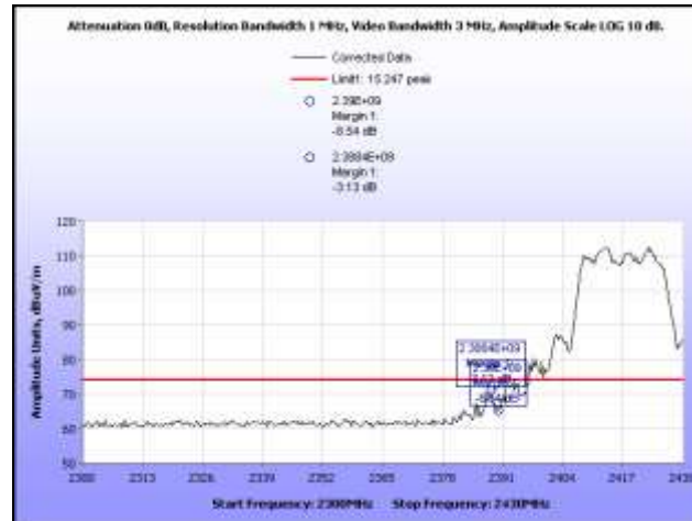
Plot 424. Radiated Band Edge, 802.11n HT20, Channel 2, 3 dBi Ceiling Mount Omni, Peak, 2.4 GHz
