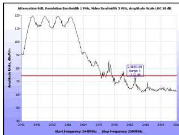
Plot 364. Radiated Band Edge, 802.11n HT20, Channel 9, 6 dBi Omni, Peak, 2.4 GHz
