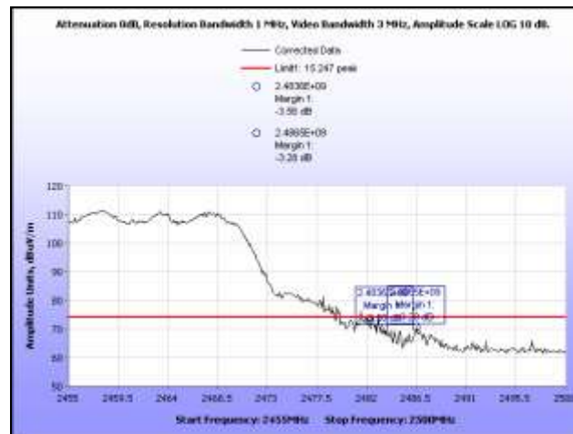
Plot 428. Radiated Band Edge, 802.11n HT20, High Channel, 3 dBi Ceiling Mount Omni, Peak, 2.4 GHz
