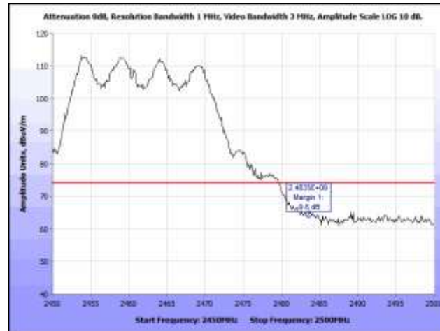
Plot 368. Radiated Band Edge, 802.11n HT20, High Channel, 6 dBi Omni, Peak, 2.4 GHz
