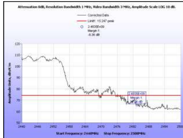
Plot 438. Radiated Band Edge, 802.11n HT40, Channel 6, High Band, 3 dBi Ceiling Mount Omni, Peak, 2.4 GHz
