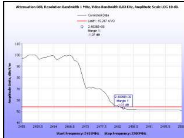
Plot 427. Radiated Band Edge, 802.11n HT20, High Channel, 3 dBi Ceiling Mount Omni, Avg., 2.4 GHz
