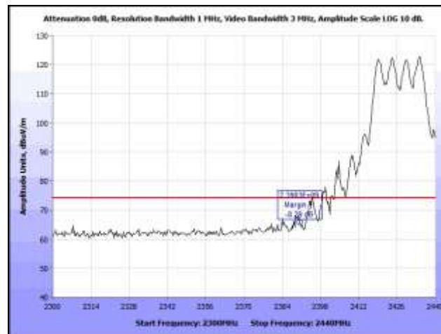
Plot 360. Radiated Band Edge, 802.11n HT20, Channel 4, 6 dBi Omni, Peak, 2.4 GHz
