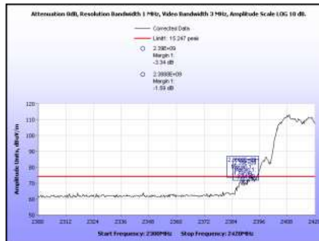
Plot 416. Radiated Band Edge, 802.11g Low Channel, 3 dBi Ceiling Mount Omni, Peak, 2.4 GHz
