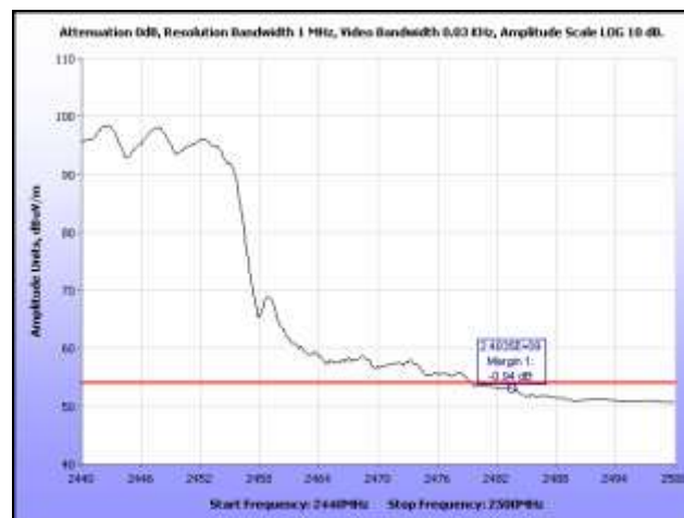
Plot 437. Radiated Band Edge, 802.11n HT40, Channel 6, High Band, 3 dBi Ceiling Mount Omni, Avg., 2.4 GHz
