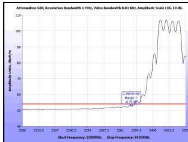
Plot 357. Radiated Band Edge, 802.11n HT20, Channel 3, 6 dBi Omni, Avg., 2.4 GHz
