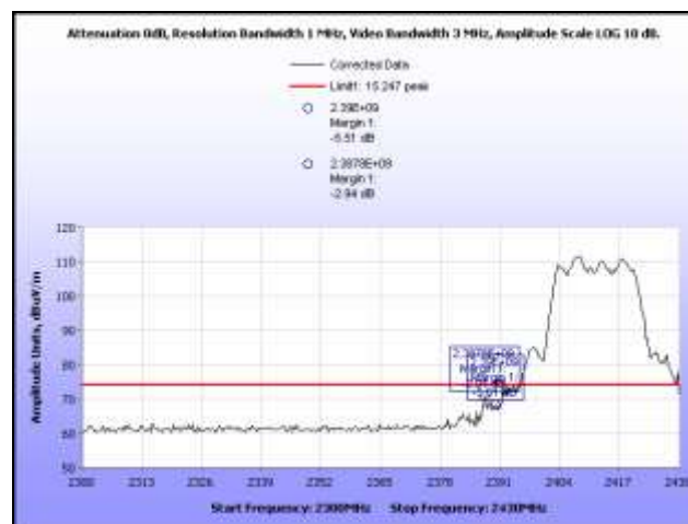
Plot 422. Radiated Band Edge, 802.11n HT20 Low Channel, 3 dBi Ceiling Mount Omni, Peak, 2.4 GHz
