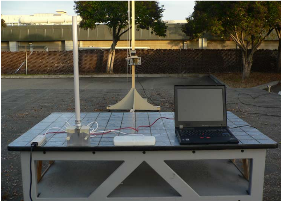
Radiated Emission – Rear View (MaxRad Dualband ( 6 dBi ))
