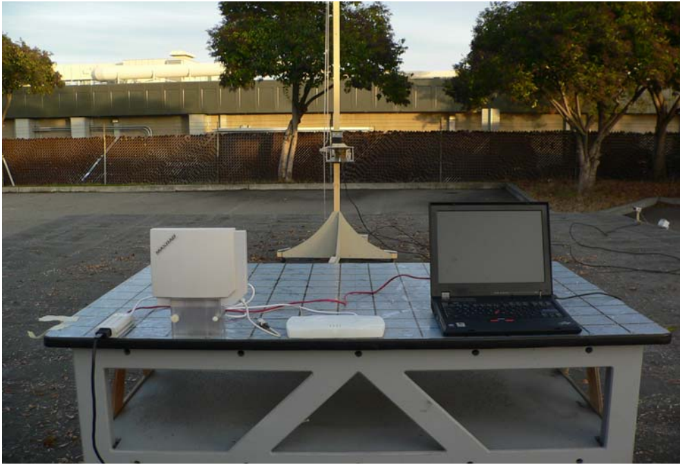
Radiated Emission – Rear View (MaxRad Antenna 2.4 to 2.5 Ghz ( 13 dBi ))
