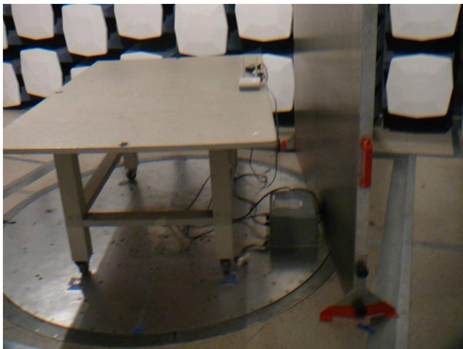
**15.3 Radiated Emission Front View (AP1010e)**
