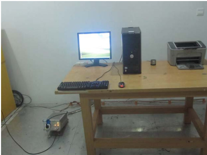
Photo of Setup for Conducted Emission Test
