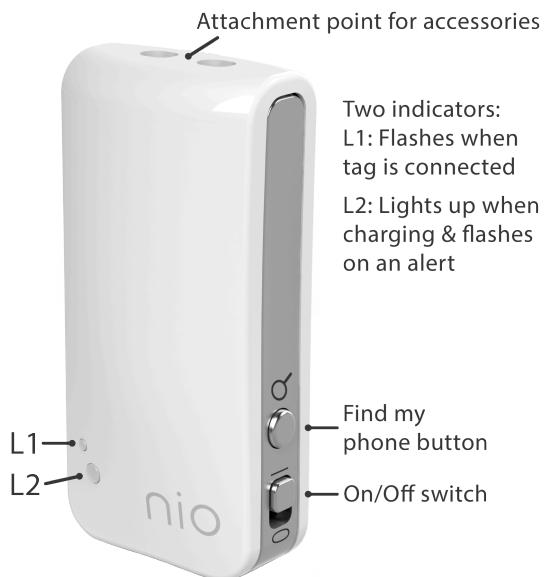
Before you can start using the nio security tag, you must fully charge the battery.
