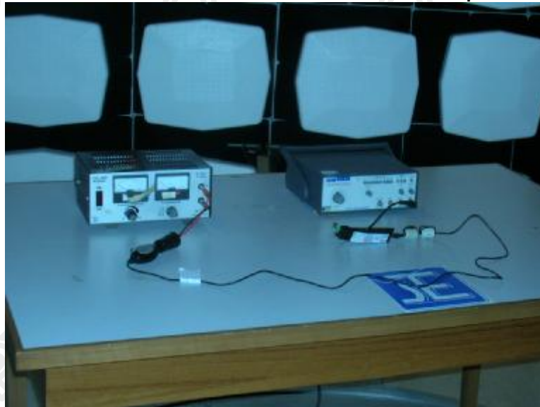
Measurement of Radiated Emission Test Set Up
