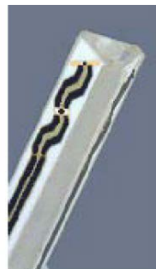
Figure 2.3 Probe Thick-Film Technique
