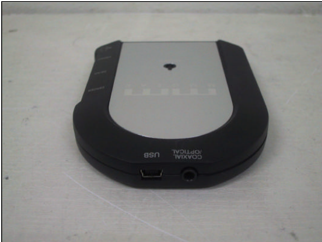
Rear of EUT
