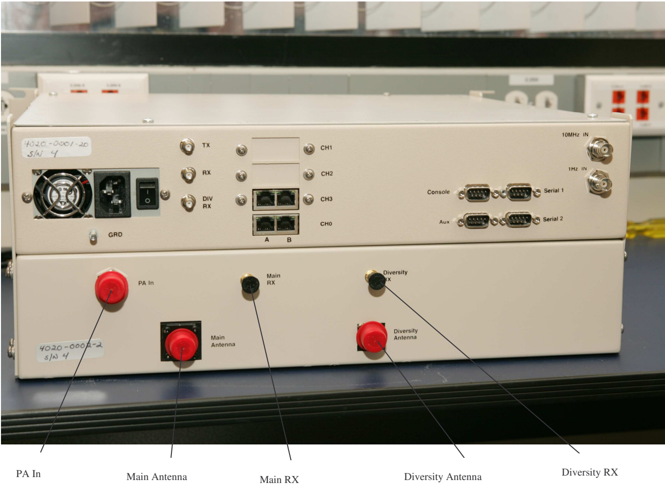
Figure 10: Protium Rear View Connections
