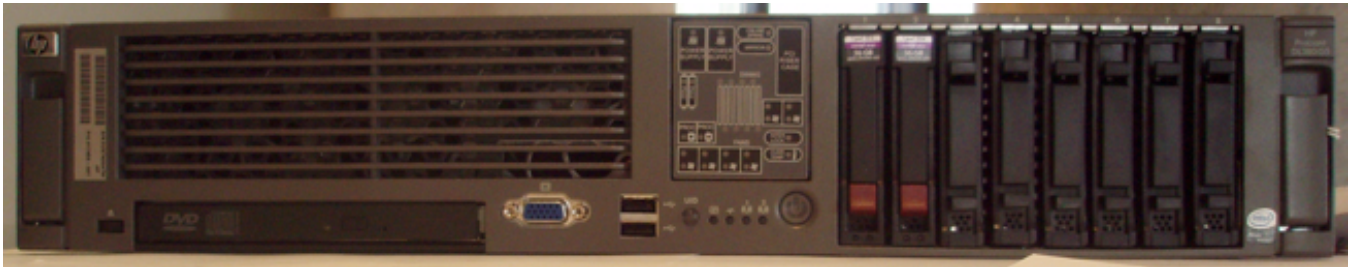
Figure 2.1: A HP ProLiant DL380 G5 Server, Front View
