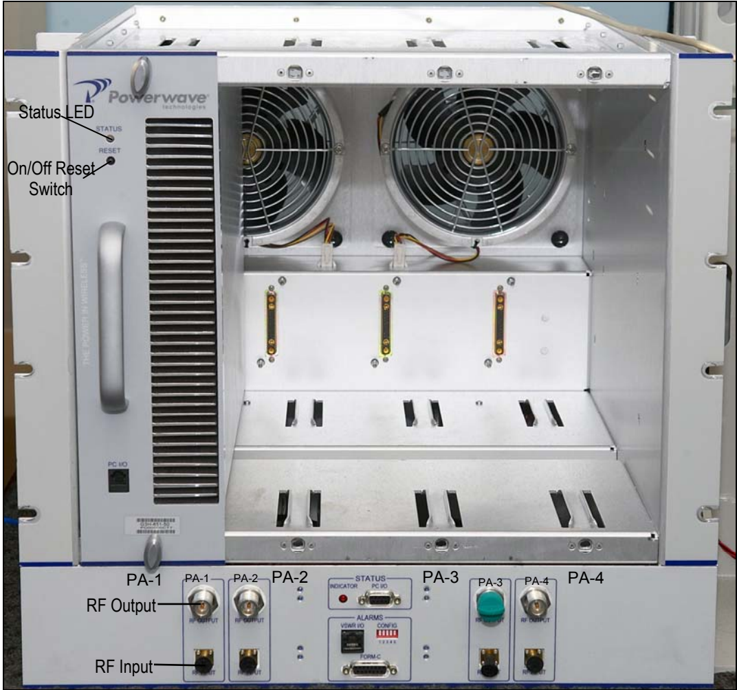
Figure 10: Powerwave Amplifier, Front View
