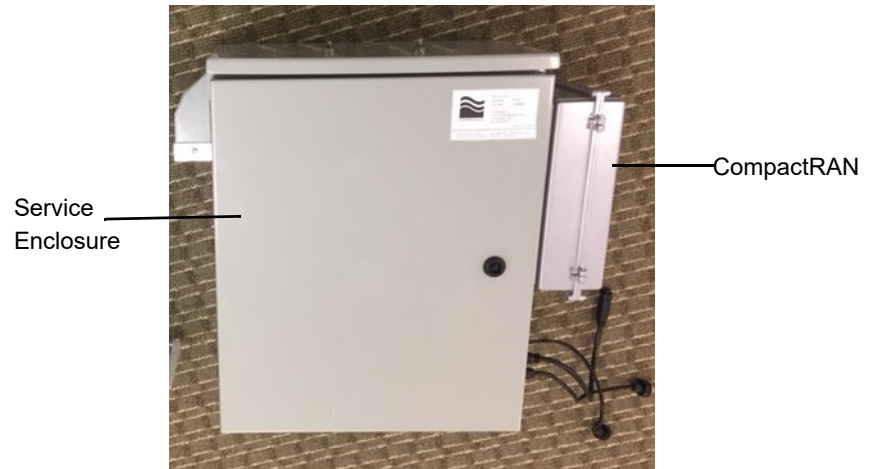
Figure 1-1. CompactRAN CDMA/GSM Base Station
