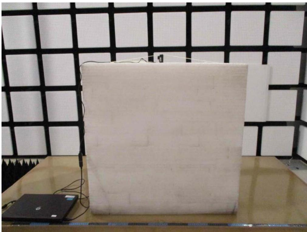
**ANTENNA PORT CONDUCTED RF MEASUREMENT SETUP**
