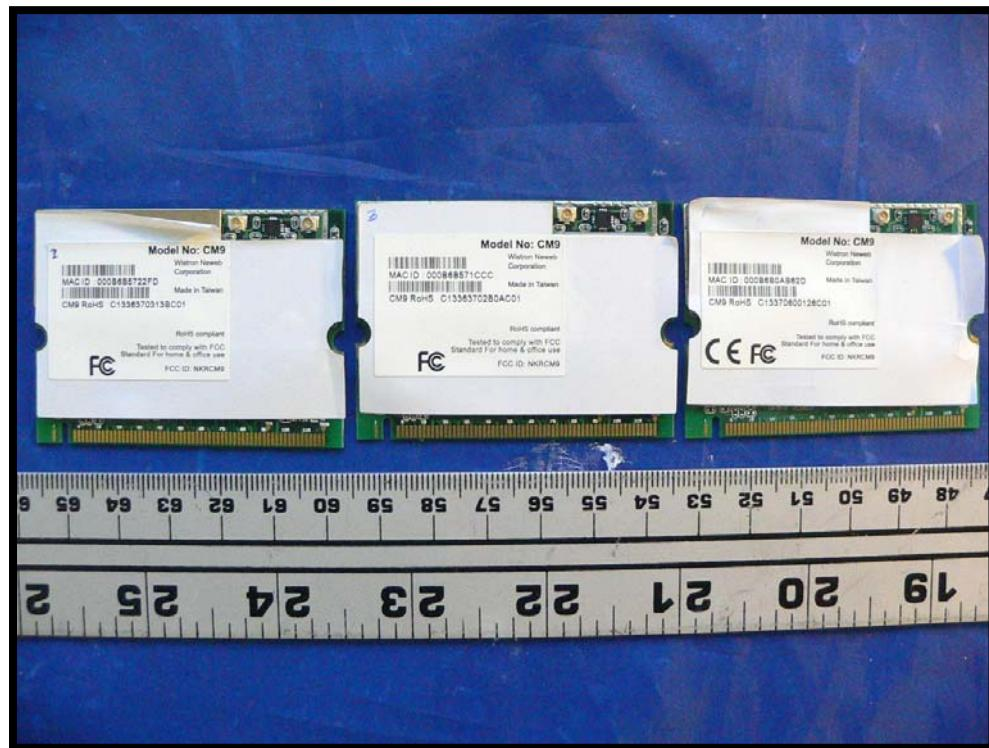
**EUT - RF Module component view with RF shield installed**
