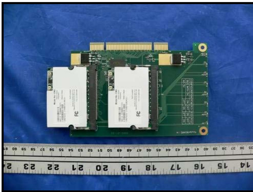
**EUT- Encryption Board with Network Board Solder View Installed On Carrier Board**
