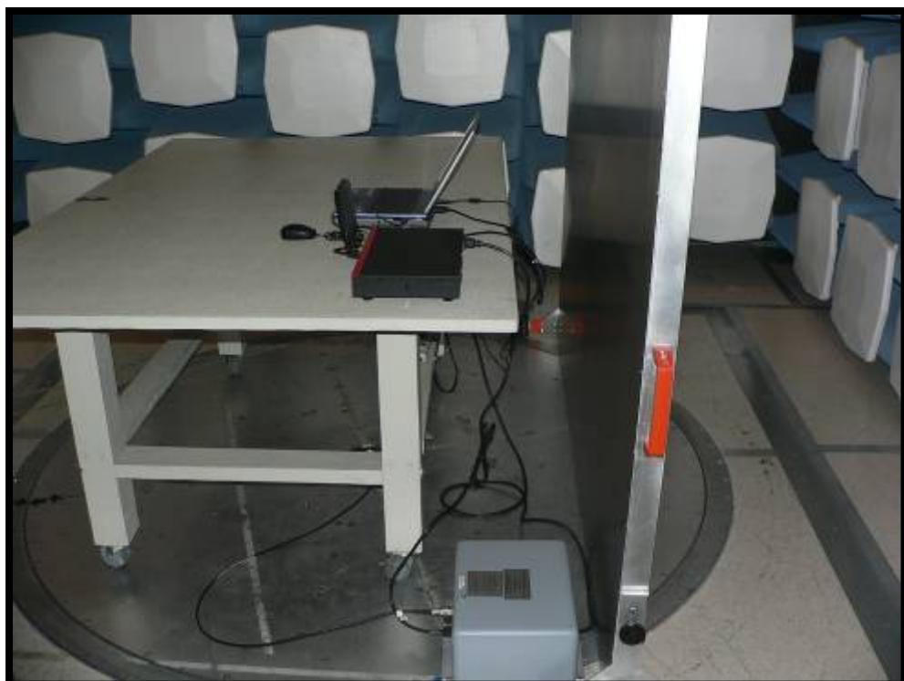
**Radiated Emissions - Front View**
