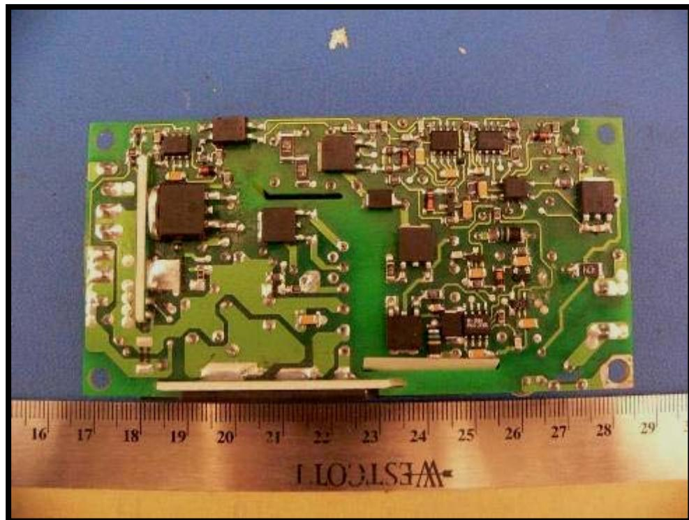
**EUT- Power Supply Sub Circuit 3 Cover off View**
