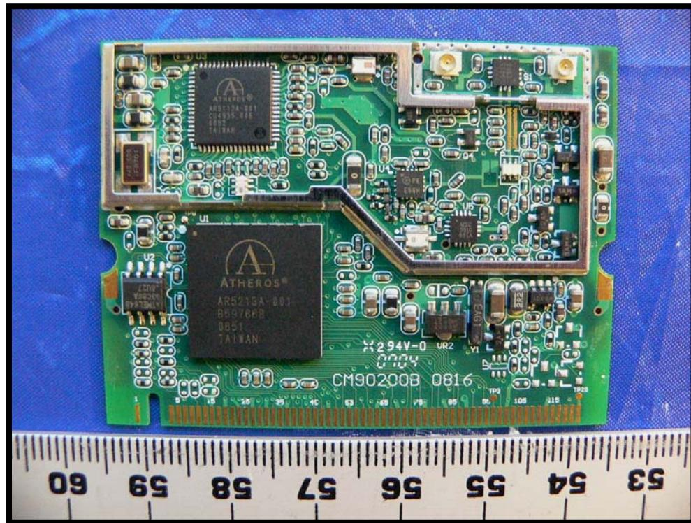
**EUT - RF Module solder view**
