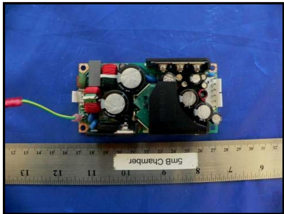
**EUT- Power Supply Sub Circuit 3 Solder View**
