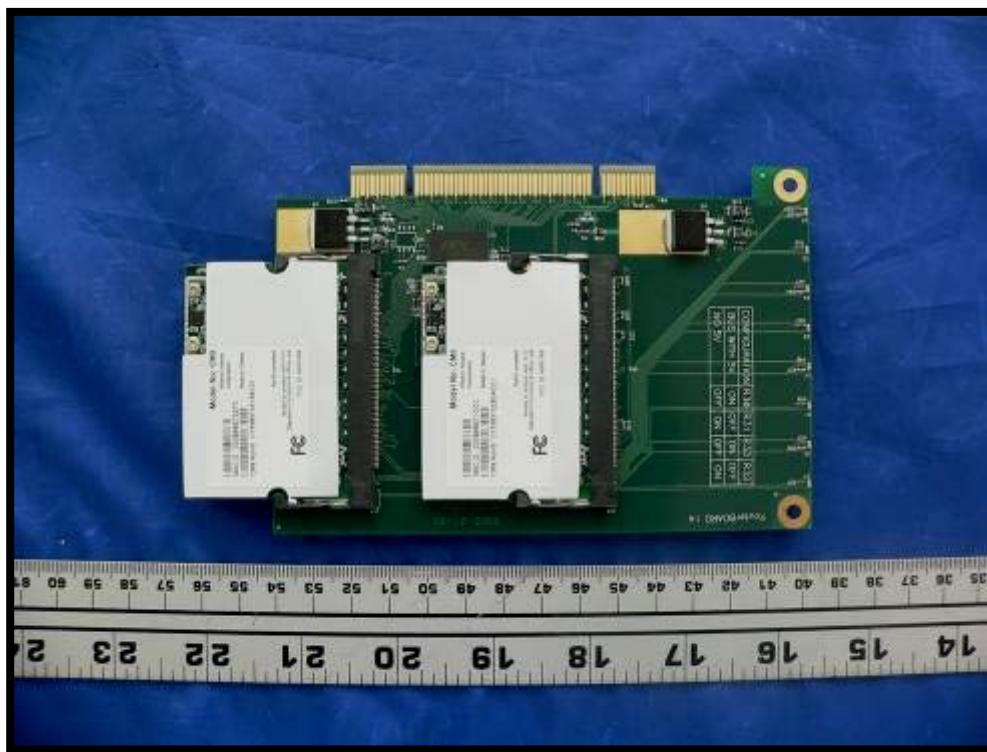
**EUT- Encryption Board with Network Board Solder View Installed On Carrier Board**
