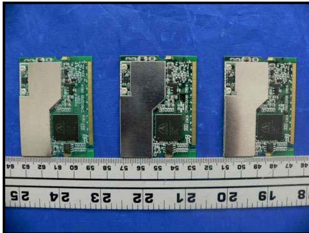
**EUT - RF Module component view with RF Shielding Removed**
