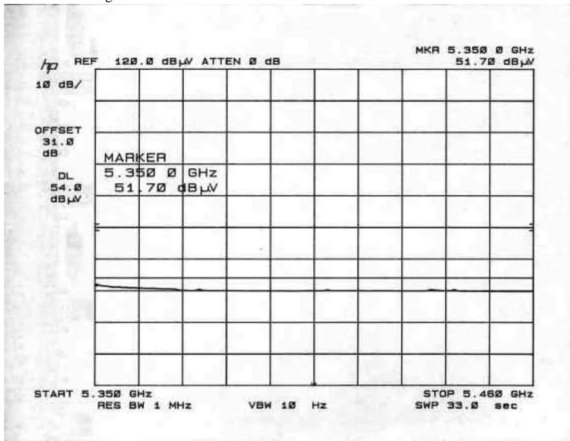
**HARMONIC AND SPURIOUS RADIATED EMISSIONS (NORMAL MODE)**
