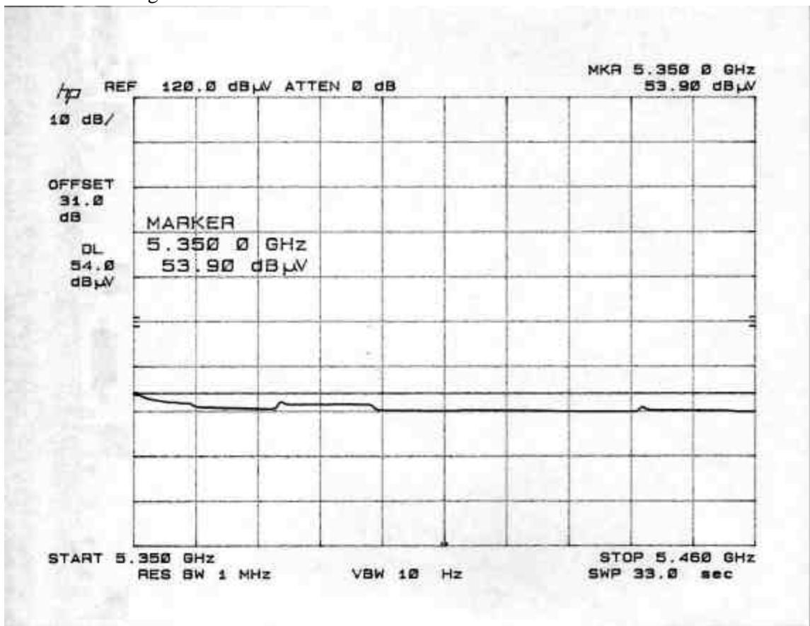
**RESTRICTED BAND RADIATED EMISSIONS (TURBO MODE, HORIZONTAL POLARIZATION)**
