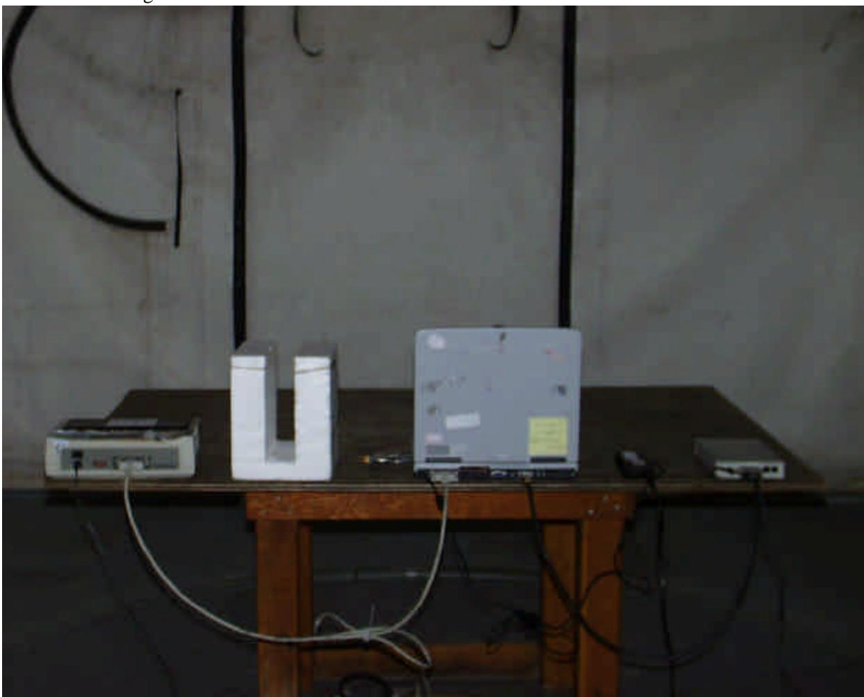
**POWERLINE CONDUCTED EMISSIONS MEASUREMENT SETUP**
