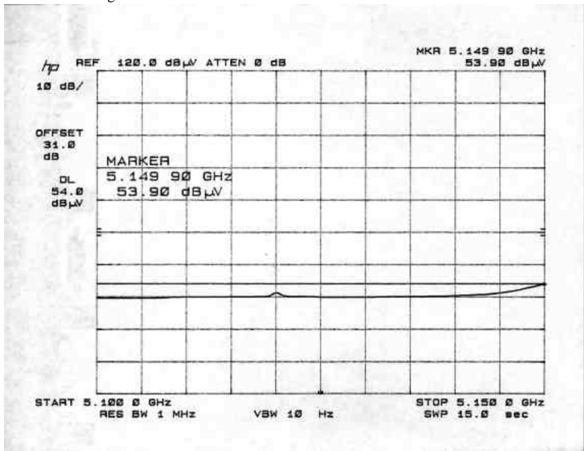
**RESTRICTED BAND RADIATED EMISSIONS (NORMAL MODE, HORIZONTAL POLARIZATION)**
