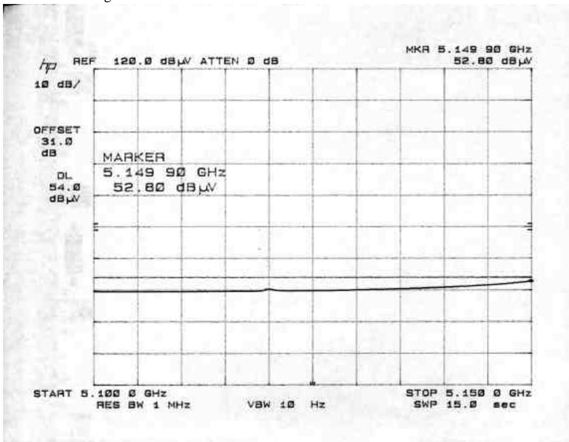
**RESTRICTED BAND RADIATED EMISSIONS (NORMAL MODE, VERTICAL POLARIZATION)**
