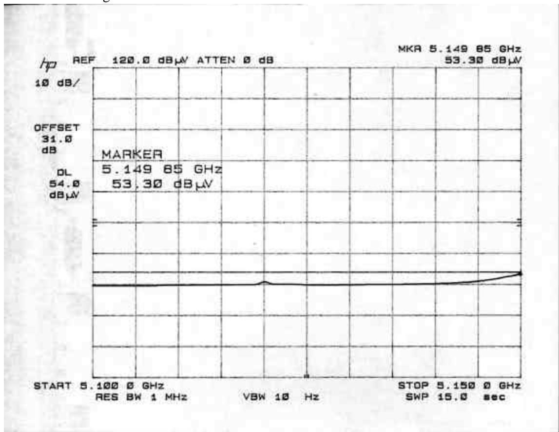
**RESTRICTED BAND RADIATED EMISSIONS (TURBO MODE, VERTICAL POLARIZATION)**
