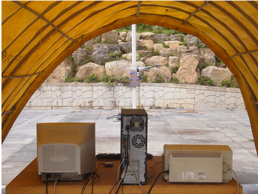
Photograph 1 : Setup for radiated Emissions
