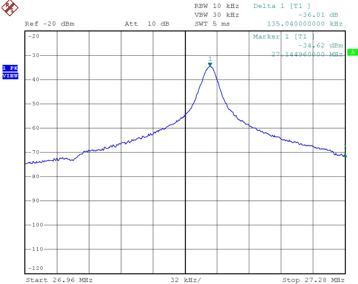
Bandedge Plot – Pursuant to FCC Part 15 Section 15. 227 Requirement      (Pass)
