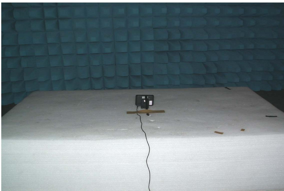
**POWERLINE CONDUCTED EMISSIONS SETUP PHOTOS**
