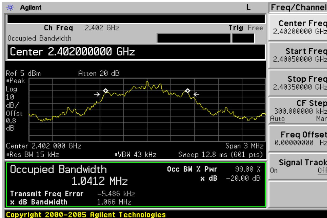
**20dB Band Width Test Data CH-Mid (EDR mode)**
