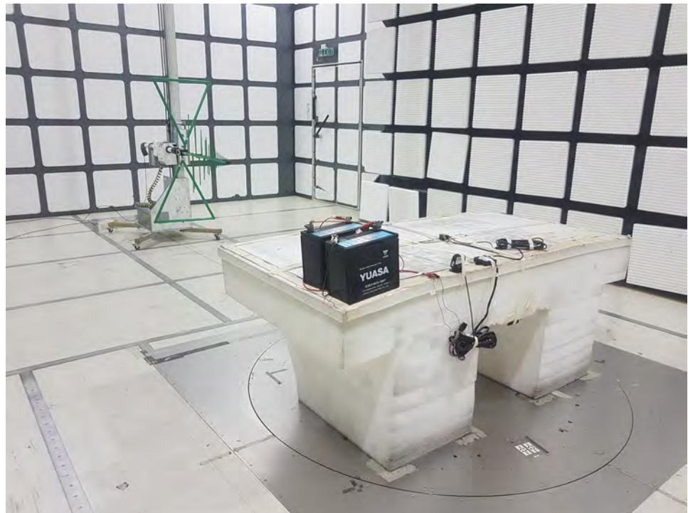
**Test Configuration: 1GHz~40GHz**
