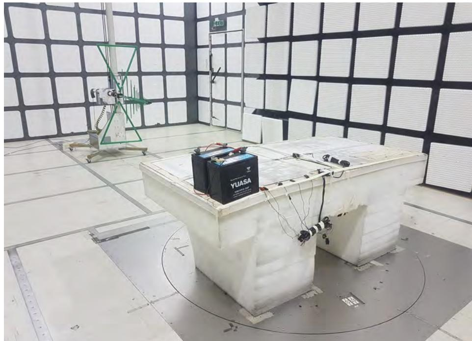
**Test Configuration: 1GHz~40GHz**
