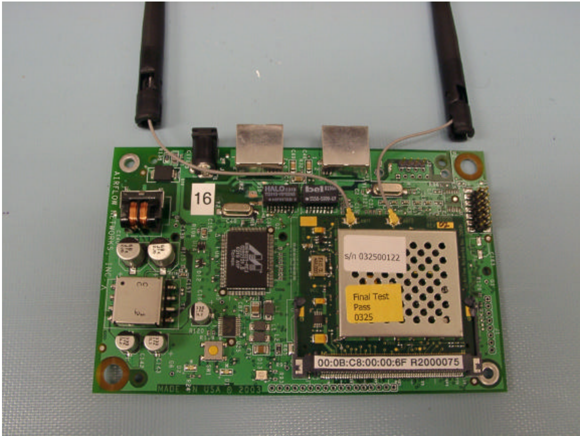
Close-up showing the Mini PCI card and connections to the antennas
