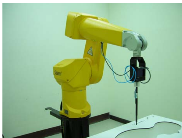
Fig. 5.2 Probe setup on robot
