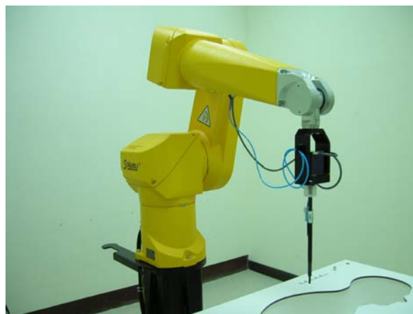
Fig. 5.2 Probe setup on robot
