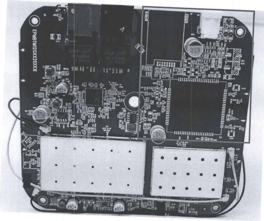
Since LTE circuit are located in an isolated block with all RF circuits shielded and have its own independent antenna, so, no big impact on the 2.4G, 5G non-license circuit is expected. We have performed spot checks on the following items to verify that if any unexpected RF conducted power or emission changes can be noted. The test results show that all spot check data are within the instrument measurement uncertainty and data reuse is justifiable.
