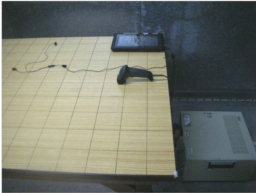
Conducted Emissions Test Setup (Front View)
