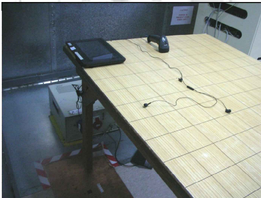
Conducted Emissions Test Setup (Rear View)
