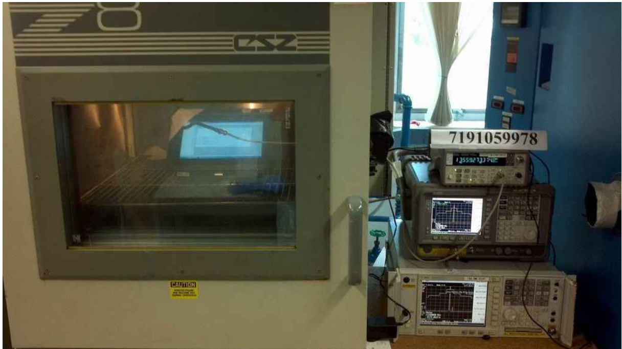
Frequency Stability Versus Temperature Test Setup
