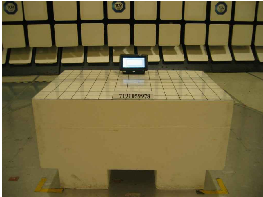
Radiated Emissions Test Setup (Front View)
