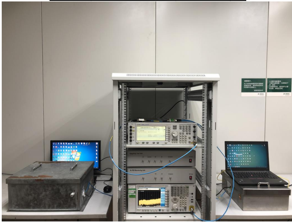
DFS Set-up Photo: Slave and Spectrum Analyzer
