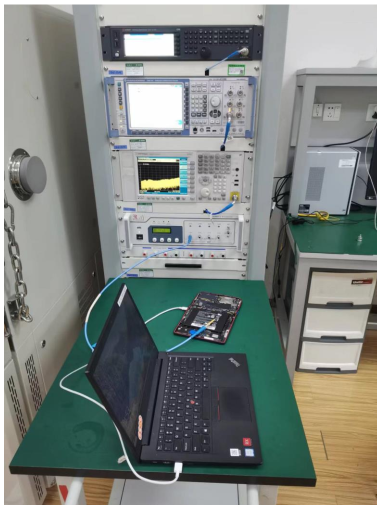
DFS Set-up Photo: Slave and Spectrum Analyzer
