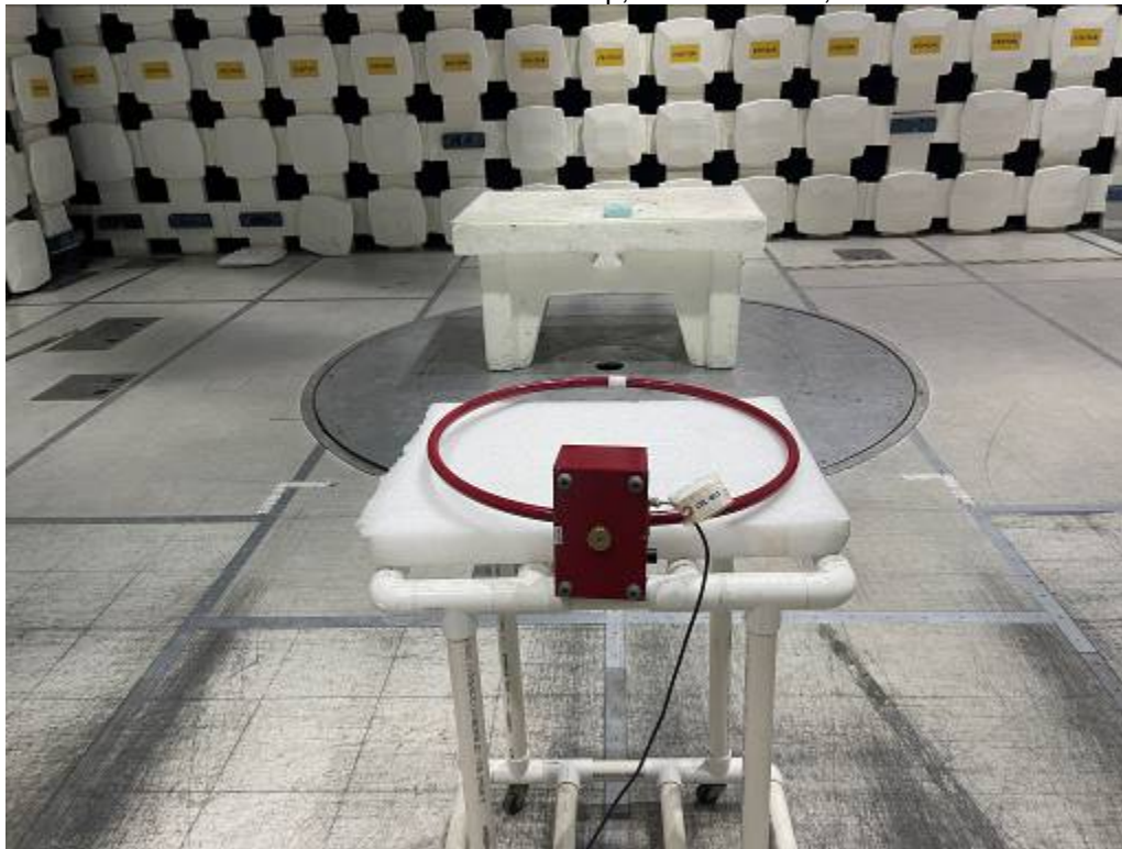
Radiated Emissions Test Setup, 9 kHz-30 MHz, Z-Axis
