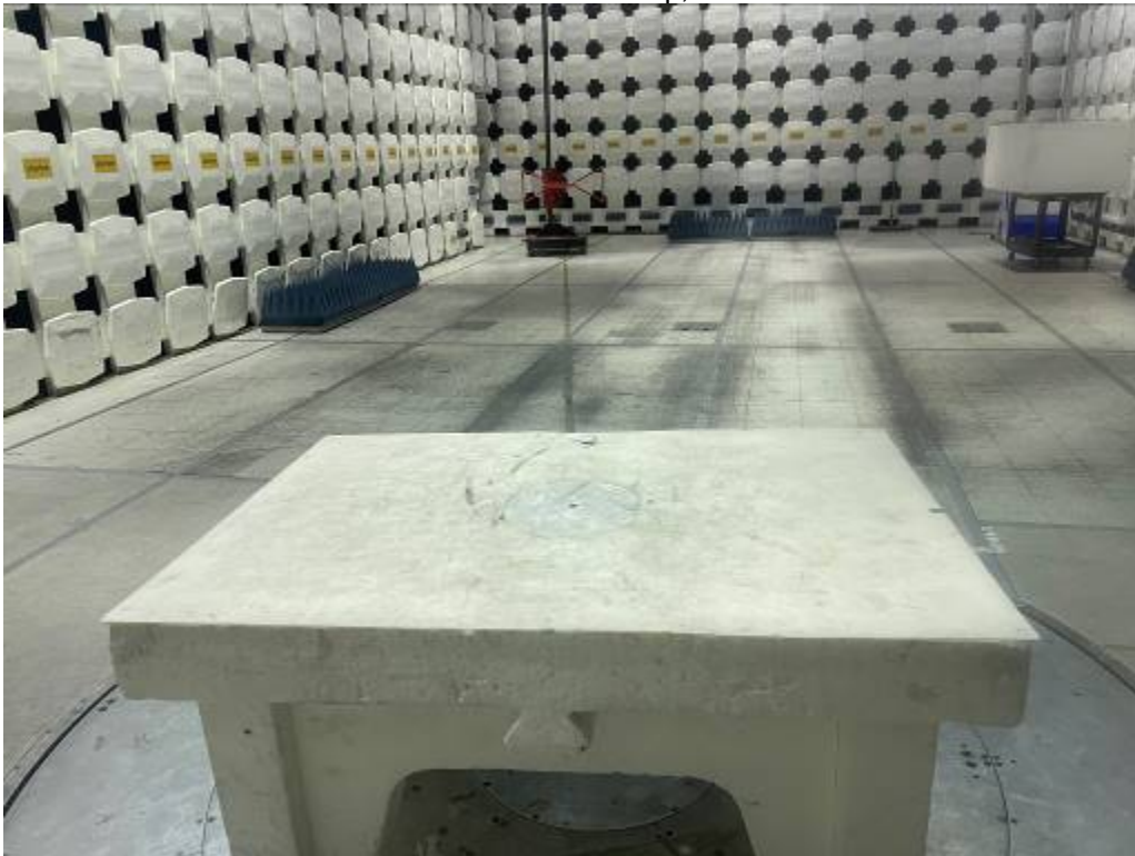
Radiated Emissions Test Setup, 30-1000 MHz
