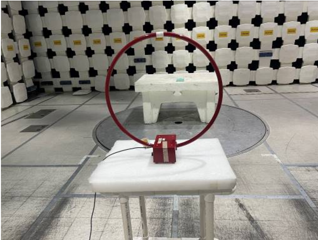
Radiated Emissions Test Setup, 9 kHz-30 MHz, X-Axis
