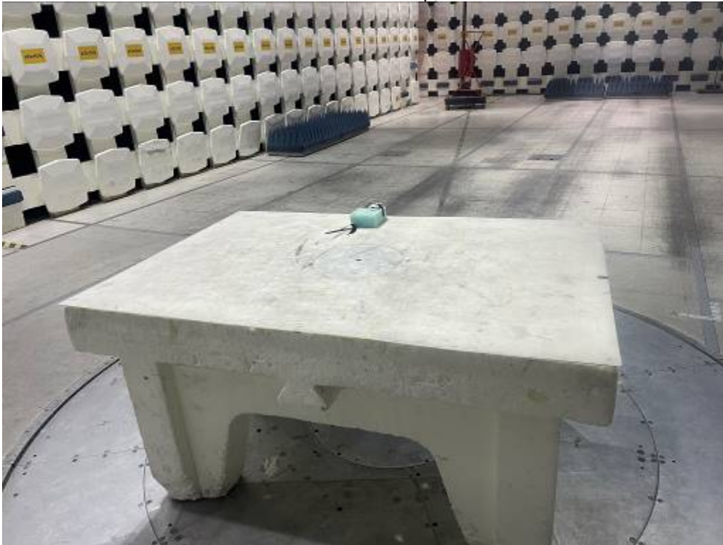
Radiated Emissions Test Setup, 30-1000 MHz
