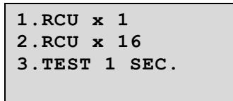
In this screen you can assign an address (group number and RCU number) to each RCU and also check the communication between the TU and RCUs.
