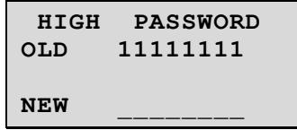
In this screen you can set the High level password. The factory default setting for High level password is 11111111.
