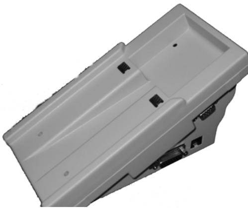
The base unit accommodates the terminal unit. The communication between the TU and the Base Unit is through mating connectors on the back of the TU and on the top of the BU. An external PTT is connectable to the side of the BU. External power can be connected to the BU by a regulated AC-DC adaptor connected to 120VAC 60 Hz input, providing to the BU its 7.5 VDC 500mA output.
