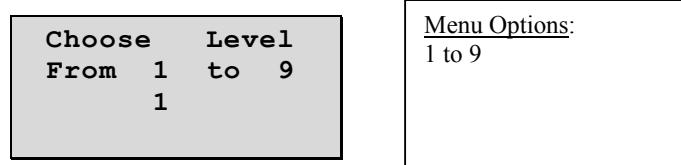
In this screen, you can set the display intensity. Select the desired intensity level between 1 to 9 and press **Enter**.
