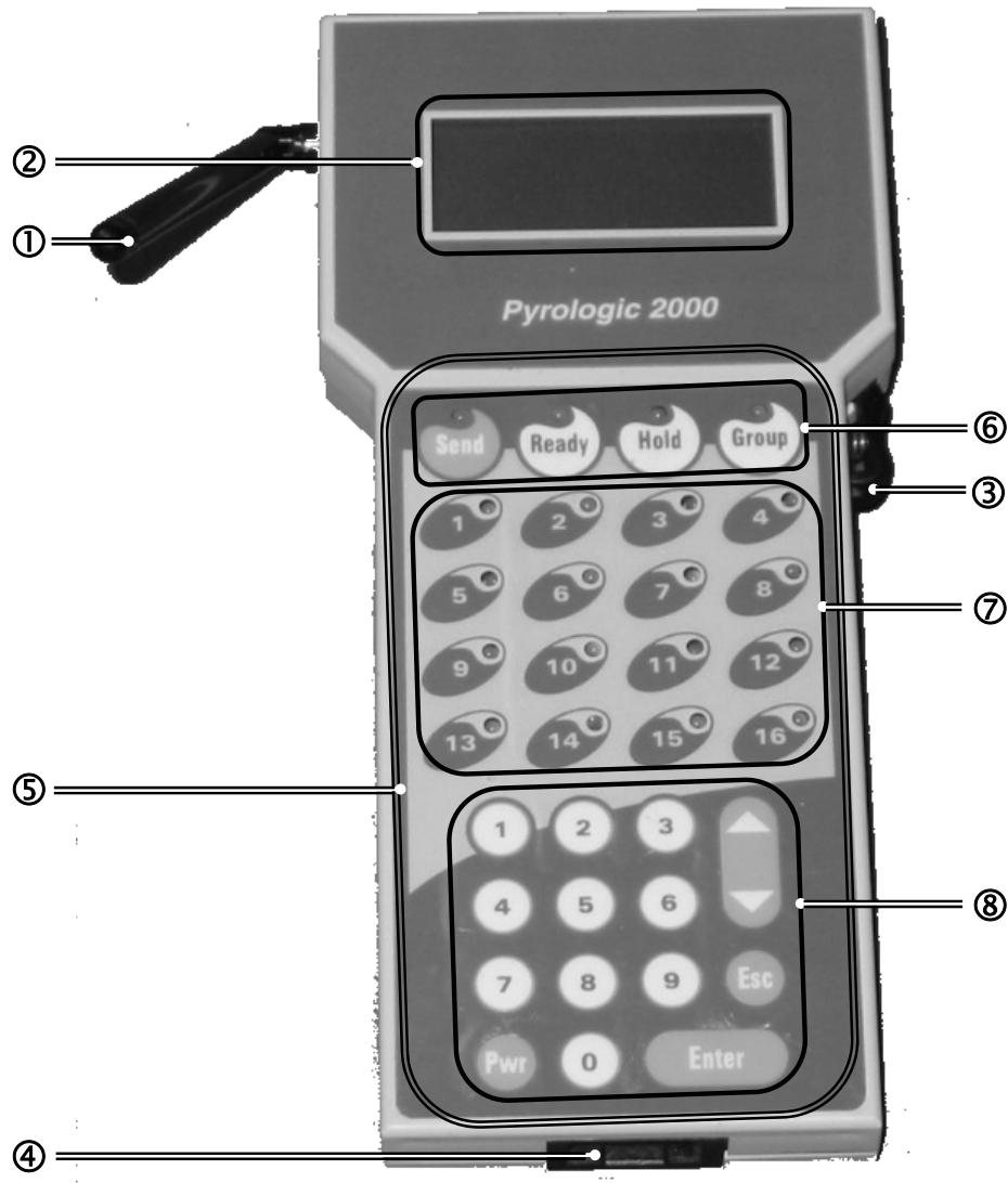
① **Foldable Antenna** - used for wireless communication with the RCUs.
