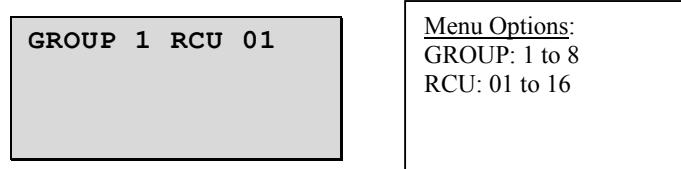
In this screen, you can assign to each RCU device a **GROUP** number and an **RCU** number. For details, see "Setting the RCU devices" on page 26.
