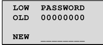
In this screen you can set the Low level password. The factory default setting for Low level password is 00000000. Note that with Low level password you cannot access the **PROGRAM EVENT** and the **CLEAR EVENT** screens.
