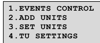
From this screen, you can access all the menus and functions of the system for programming and setting events, adding and setting RCUs, and setting the system environment such as passwords, display brightness, clock etc.
