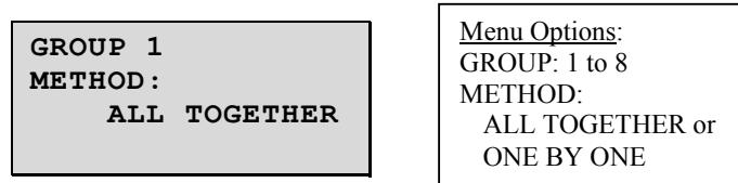
In this screen, you can assign to each RCU X 16 device a **GROUP** number and an **RCU** number. The RCU X 16 works as 16 different RCUs in one group.
