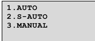
In this screen you can select the active event mode (AUTO, S-AUTO or AUTO) for programming, firing, or clearing. For each event you can program or choose Manual and/or Semi-automatic and/or Automatic mode.
