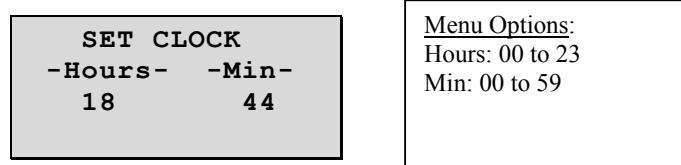
In this screen, you can set the time. Setting the time is particularly important when setting the alarm.
