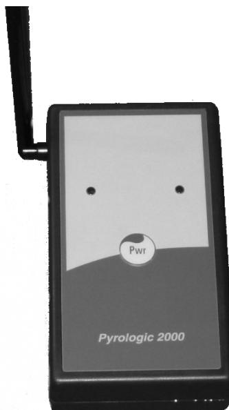
The Extension Unit (XU) has one key, 2 LEDs, RJ11 connector, Antenna and TRI-POD mount.
