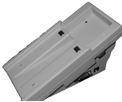
The base unit accommodates the terminal unit. The communication between the TU and the Base Unit is through mating connectors on the back of the TU and on the top of the BU. An external PTT is connectable to the side of the BU. External power can be connected to the BU by a regulated AC-DC adaptor connected to 120VAC 60 Hz input, providing to the BU its 6 :- 7.5 VDC 500mA output.
