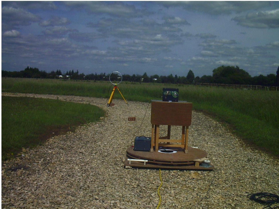
Photograph 3 Radiated Emissions on Test Jig
