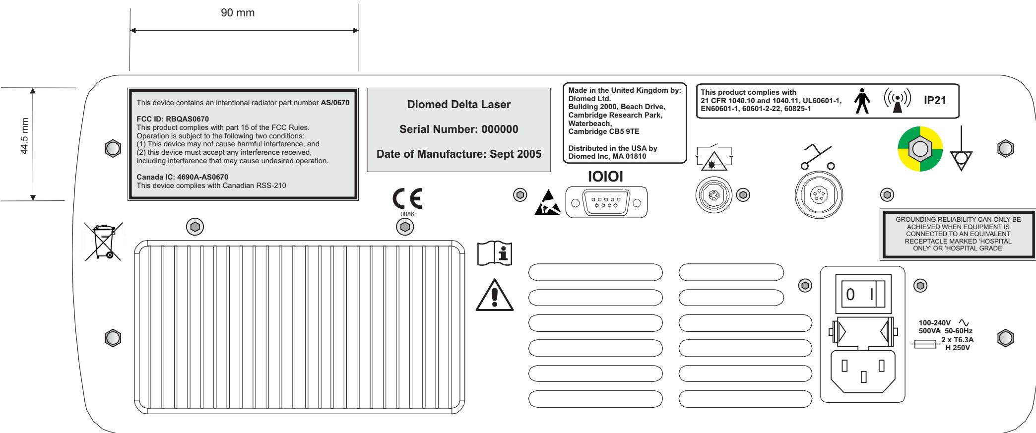
FCC / IC Label is chemical and solvent resistant polyester and attached with a permanent adhesive.
