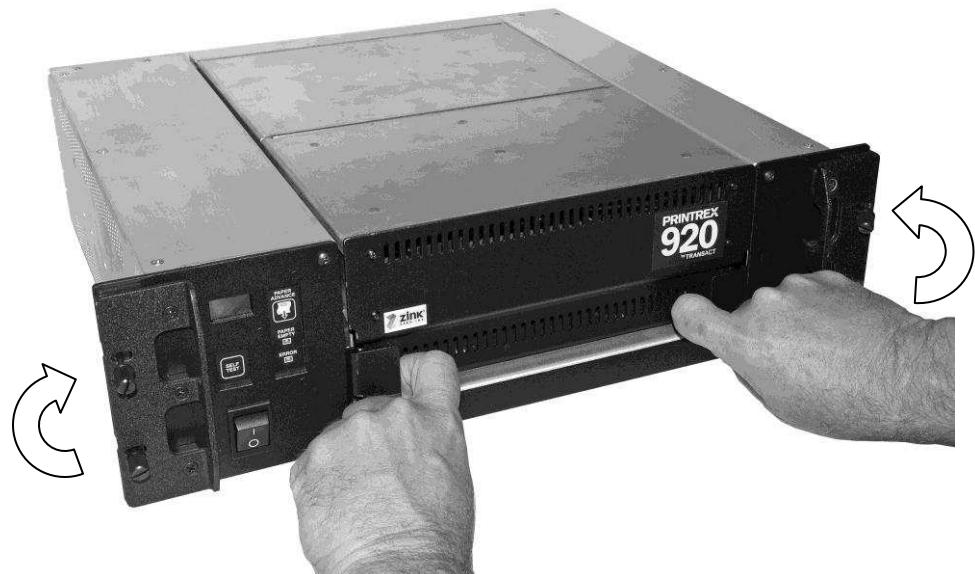
3. Rotate the upper unit upward to open the printer.
