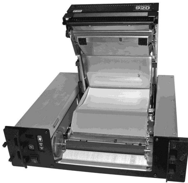
4b. Black and white thermal paper stock is loaded as a fanfold stack of paper. Lower the stack into the paper tray as shown.
