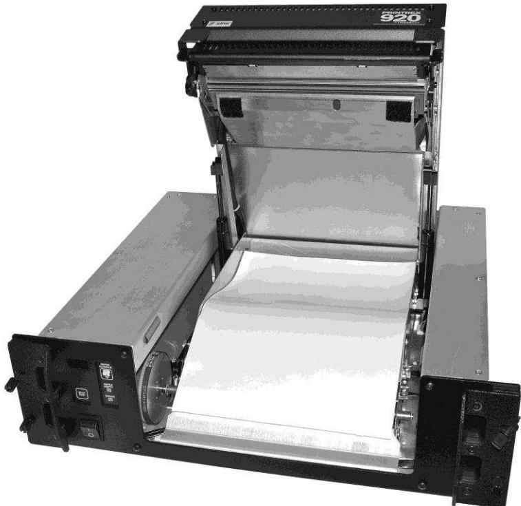
8. After loading paper, push the upper unit down until it clicks into place. Press the PAPER ADVANCE button on the front console to advance the first sheet. Slide the printer back into the rack if appropriate.
