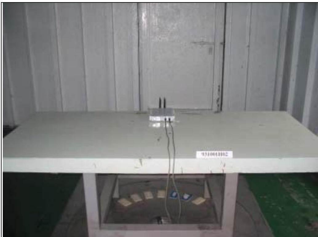
**RADIATED EMISSION TEST [Sample 2 (Internal Power)]**
