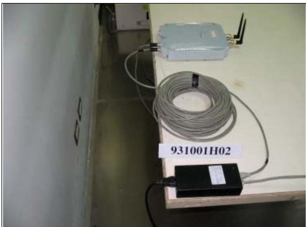
**CONDUCTED EMISSION TEST [Sample 2 (Internal Power)]**
