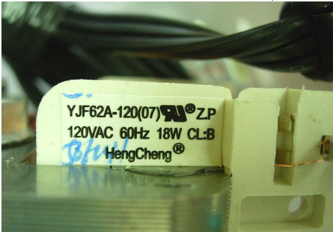
Photo 27 M/N TSK-8402AMM, Label of Fan Motor
