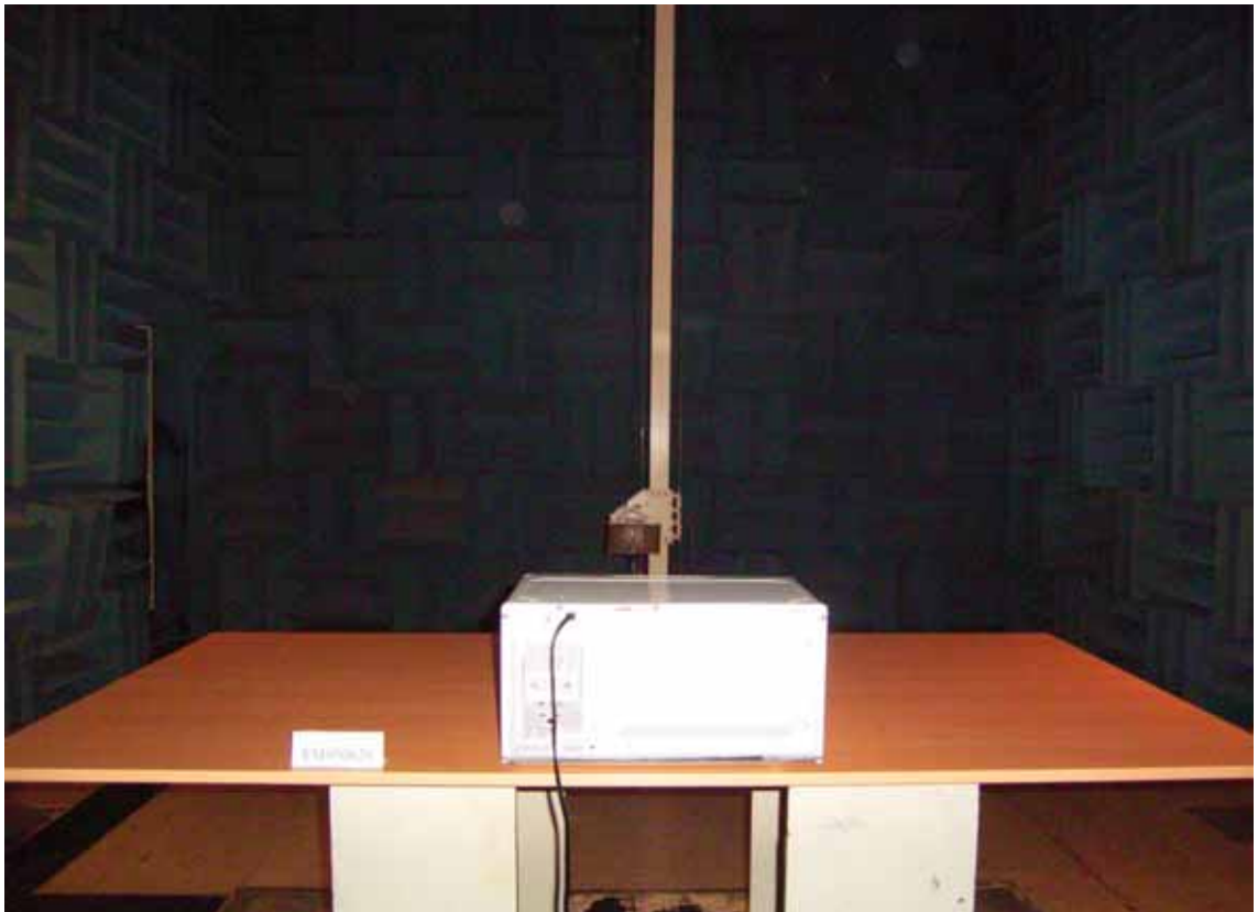
BACK VIEW OF RADIATED MEASUREMENT
