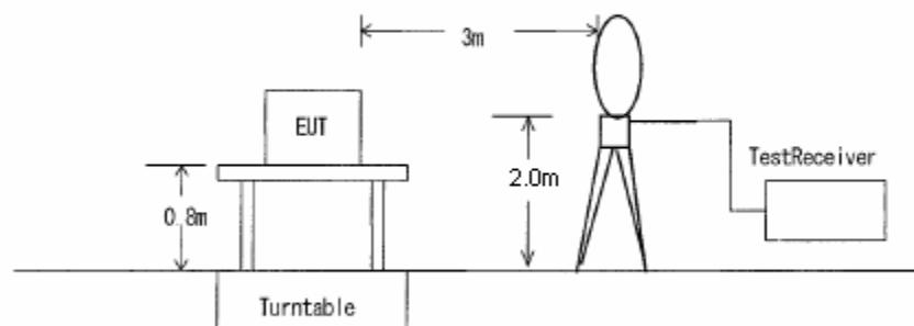
(B) Radiated Emission 30MHz - 1000MHz
