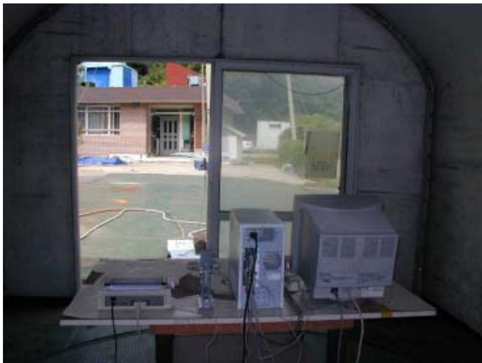
RADIATED EMISSION SETUP PHOTOGRAPH - REAR VIEW ( 300 - 1000 MHz )
