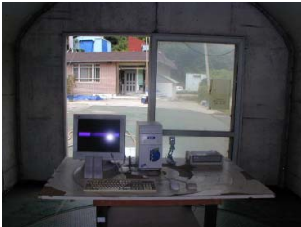
RADIATED EMISSION SETUP PHOTOGRAPH - FRONT VIEW ( 300- 1000 MHz )
